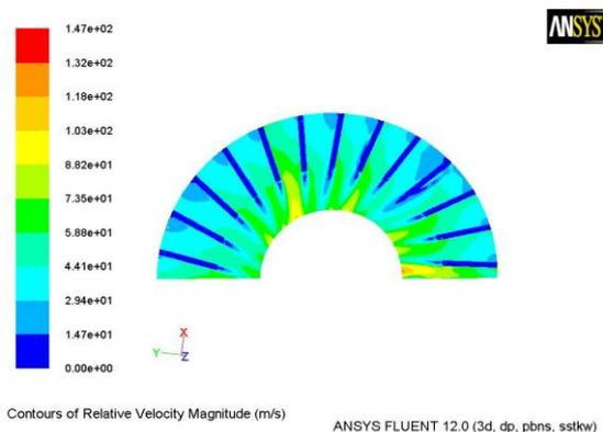
Figure VI. Relative velocity at midplane of rotor at 24rad/s
