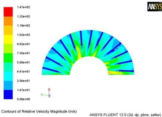
Figure VI. Relative velocity at midplane of rotor at 24rad/s
