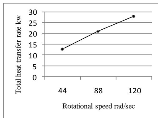
Figure IX. Total heat transfer rate as a function of rotor speed
