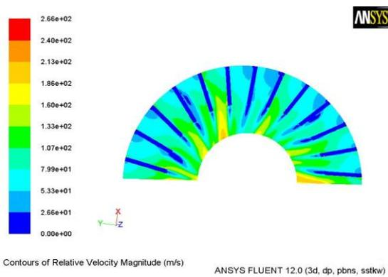
Figure VII. Relative velocity at midplane of rotor at 88rad/s
