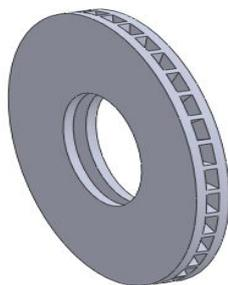
Figure II: 3D model of disc brake in solid works
