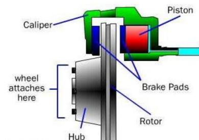
Figure I. Scheme of a disc brake
