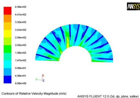
Figure VIII: Relative velocity at midplane of rotor at 120rad/s
